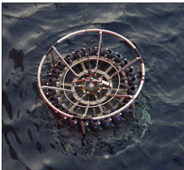
The CTD and rosette package descends into the frigid Arctic waters to retrieve more seawater samples for our hydrographic and chemical analysis. Photo by Rick Krishfield, WHOI.
