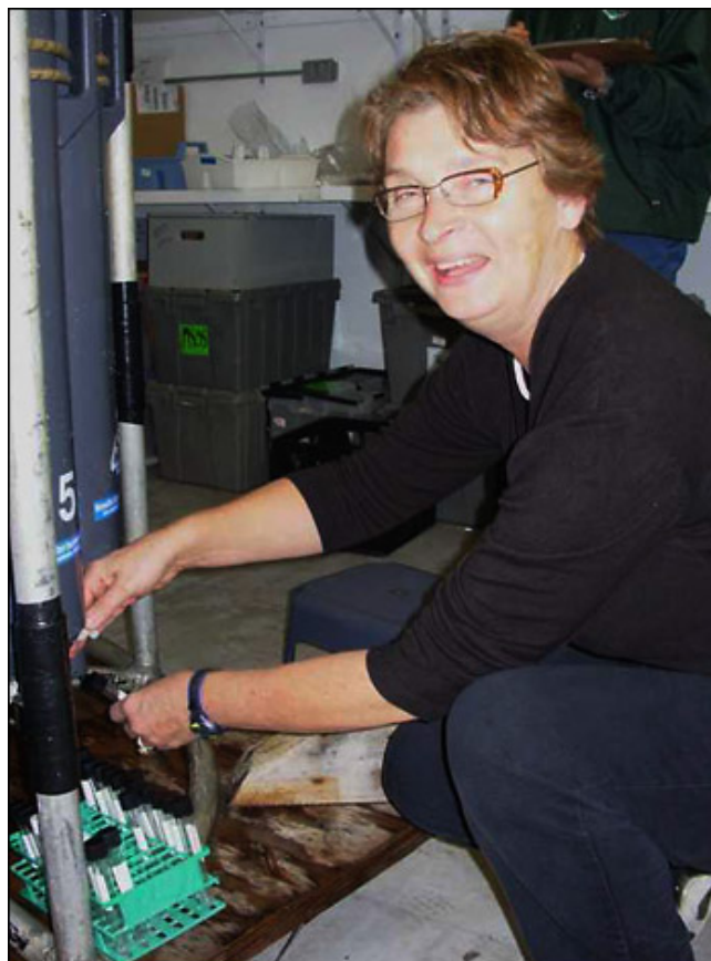
The author drawing seawater from the CTD rosette bottles for nutrient analysis. Photo by Rick Krishfield, WHOI.
