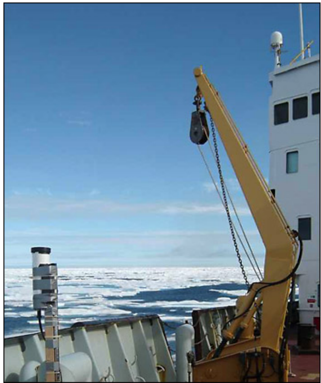
The surface optical sensor fixed at to the ship's railing near the deployment location in order to provide a reference for the profiler when lowered into the water. Photo by Jiuxin Shi, OUC.
