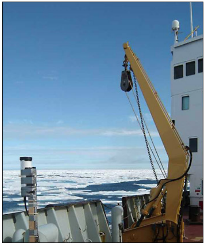
The surface optical sensor fixed at to the ship's railing near the deployment location in order to provide a reference for the profiler when lowered into the water. Photo by Jiuxin Shi, OUC.
