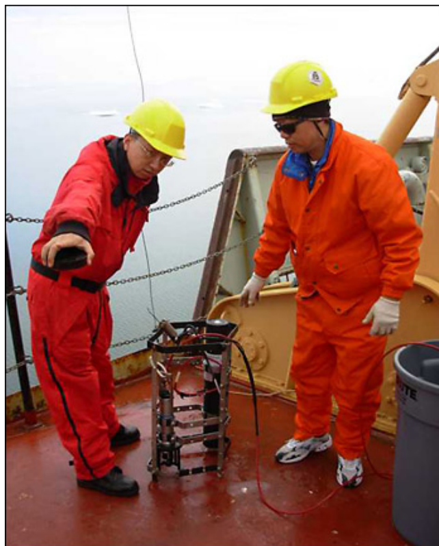
Jiuxin Shi and Yutian Jiao prepare the optical seawater profiler for deployment. The optical instrument must be lowered at the side facing the sun, and finding an appropriate opportunity with reasonable winds, sea ice, clouds sun is very important for the deployment, but can be difficult in the Arctic Ocean. Photo by Rick Krishfield, WHOI.
