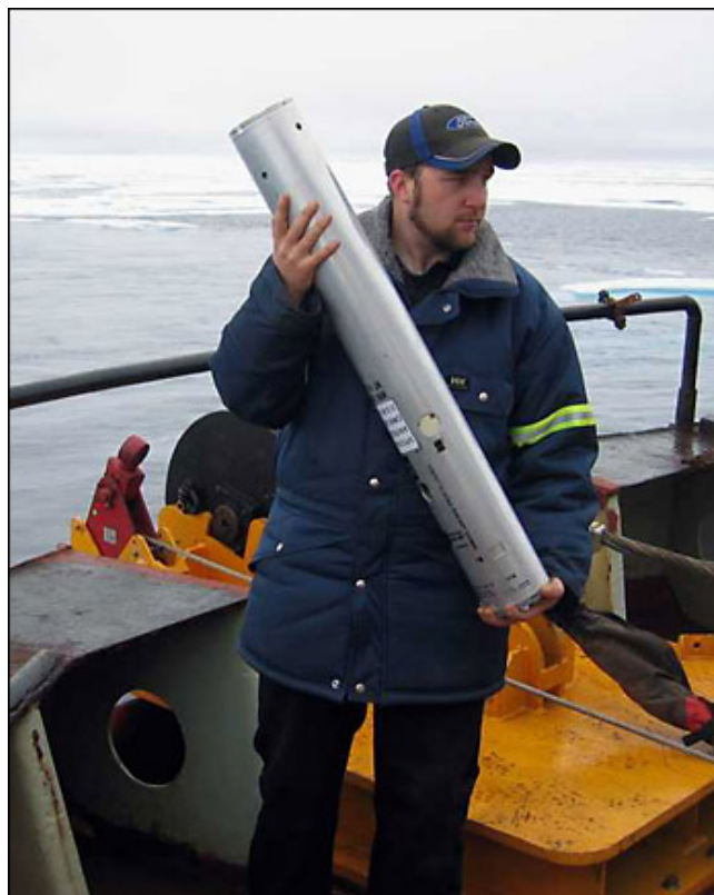
Summer student Ryan Pike (NRCan) is getting ready to deploy the sonobuoy at the stern of the Louis . A radio transmitter will relay the data back to the ship. Photo by Thomas Funck, GEUS.
