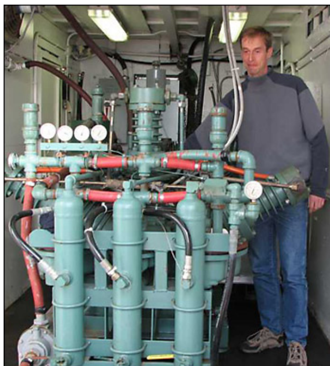
Senior scientist Thomas Funck (GEUS) in the compressor container. The compressed air (pressure of 2000 pounds per square inch) is used by the air guns to create the sound waves for the seismic experiment. Photo by Ryan Pike.
