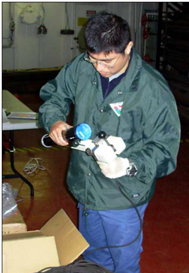
The author loads an XCTD into the hand-held launcher and then initializes the data acquisition computer program. Photo by Rick Krishfield, WHOI.
