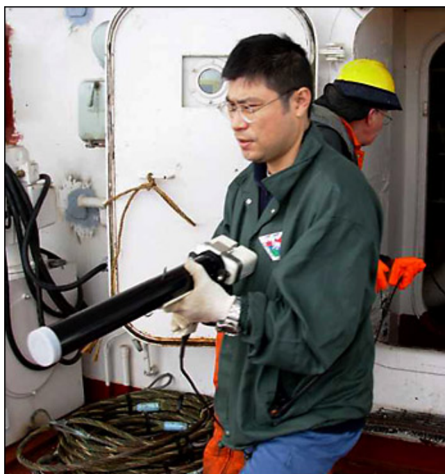
While the XCTD and launcher are carried out to the stern, Terry Rhyno feeds the serial communications cable through the passage. Photo by Rick Krishfield, WHOI.
