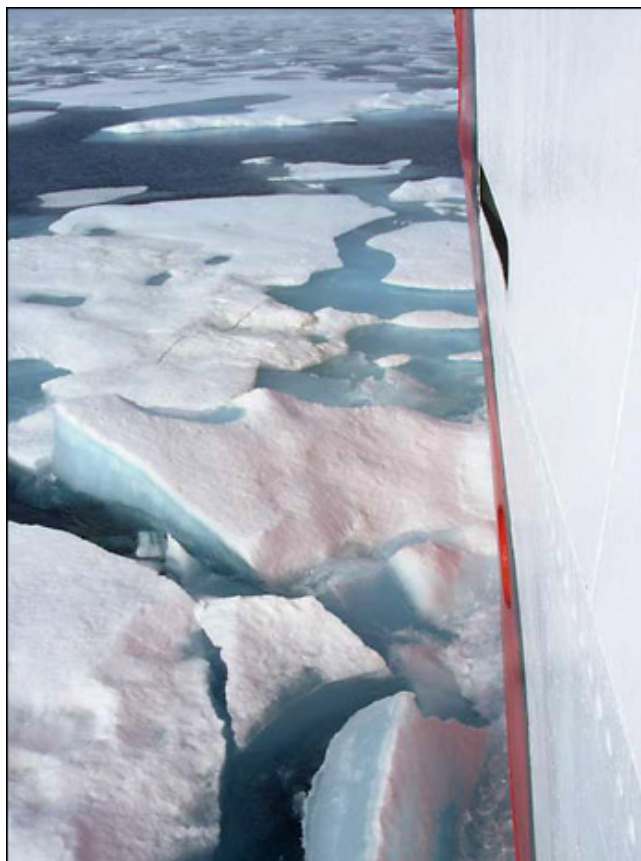
Chunks of 1 m (3 ft) thick ice are pushed effortlessly aside by the Louis .
