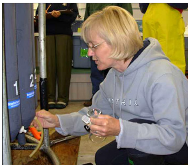
Mary Steele draws water from a Niskin bottle for oxygen analysis. Photo by Rick Krishfield, WHOI.
