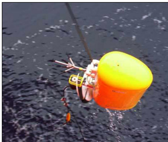
MMP profiling CTD instrument finally being recovered at the end of a long difficult mooring recovery operation. Photo by Rick Krishfield, WHOI.
