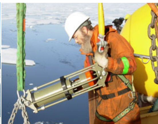
Bosun Bob Taylor, handling an acoustic current meter during the deployment of Mooring D, a few days ago.
