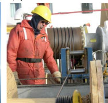
Seaman Alfie Sears is keeping an eye on the mooring wire and spooler during a mooring deployments.
