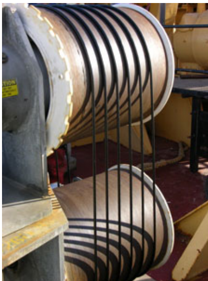
The Lebus winch is the workhorse of the mooring operations. It has been working flawlessly during this program.
