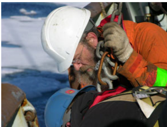
Bosun Bob Taylor and Kris Newhall are using a chain hook to transfer the load and disconnect the different instruments as we are pulling the mooring on board.
