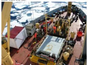
foredeck. The Lebus winch can be seen on the port side (left), transfer the load and disconnect the different instruments as and the wire goes over the side through the A-frame on the starboard side (off the picture, to the right).
