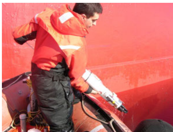
I am putting the small CTD in the water, right next to the Louis . (Photo by Jennifer Hutchings).
