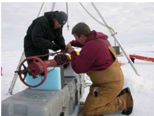
Kris Newhall and Jim Dunn are verifying the instrument package of the ocean flux buoy, just before lowering through the ice.
