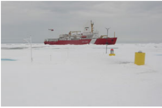
The three buoys finally installed: ice mass balance buoy, barely visible in white on the left, the wind generator and the yellow and red float of the ocean flux buoy in the center, and the ITP on the right. Time to go back!
