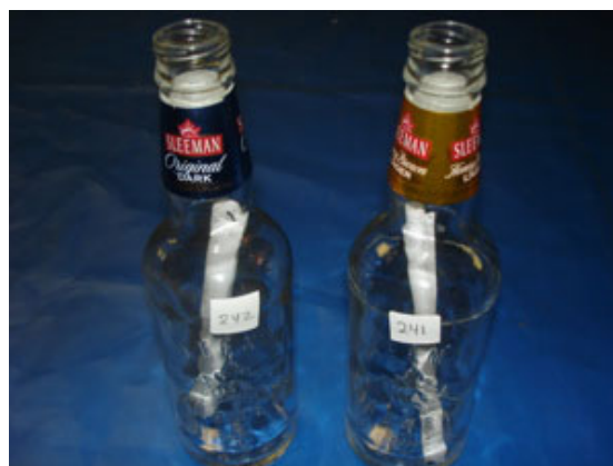
A couple of surface current tracking devices, before being sealed with a cork and wax. (Photo by Alice Orlich).
