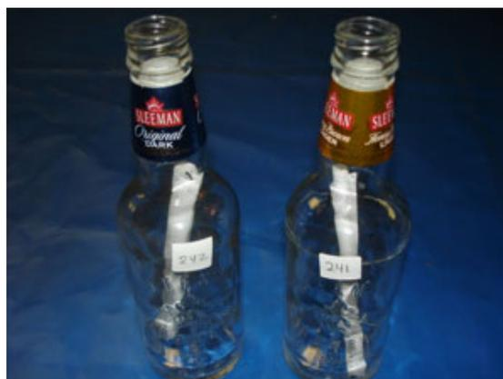
A couple of surface current tracking devices, before being sealed with a cork and wax. (Photo by Alice Orlich).
