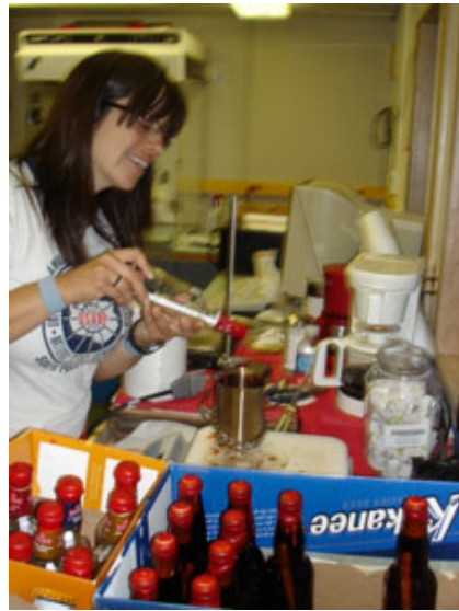
Alice is sealing the bottles by dipping them in hot wax. (Photo by Helen Drost).
