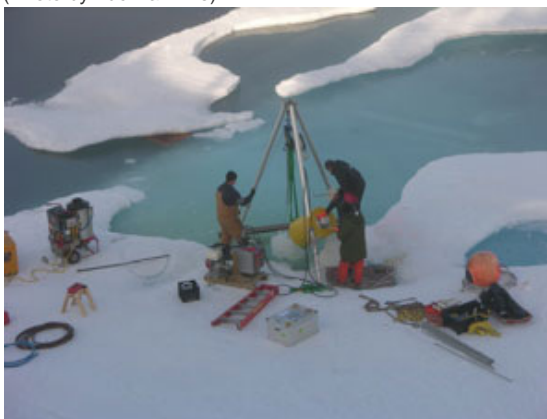
The melting operation results into a big 'ice core' with a diameter of about 2 ft. The float can be lifted... (Photo by Luc Rainville).
