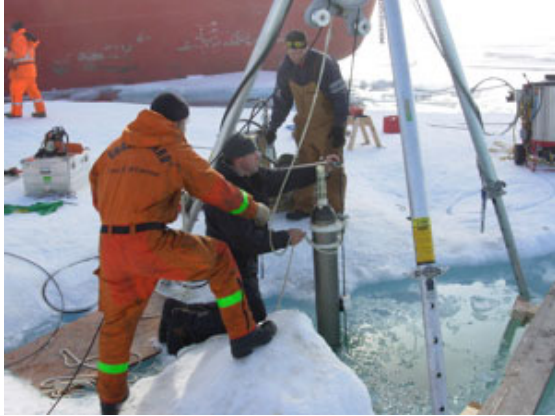
Finally come out the crawler itself and the bottom weight. (Photo by Rick Krishfield).
