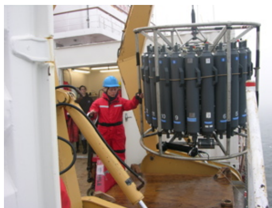
Jen has to collect her samples using the CTD rosette. Here she is helping during recovery.
