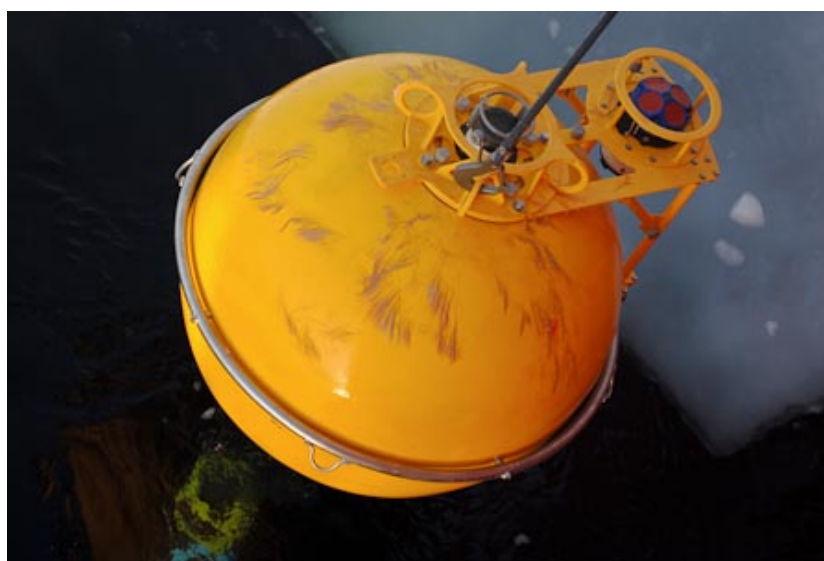
The main floatation buoy of one of the three moorings recovered during the expedition. This buoy came up covered in Arctic aquatic flora.
