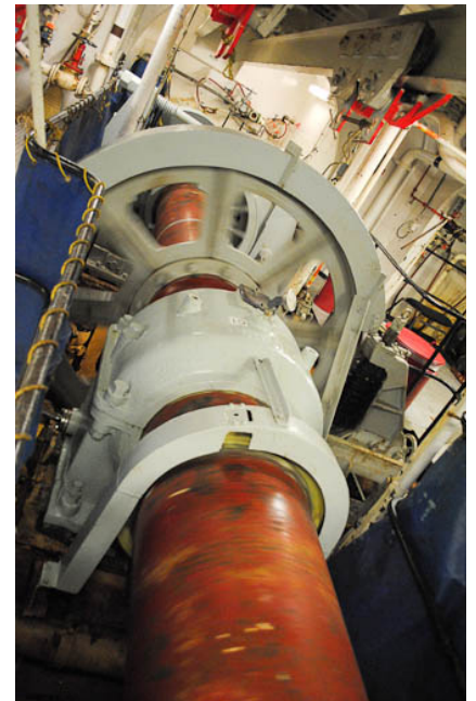
Shaft in motion. Each of the three propeller shafts is the thickness of a tree trunk.
