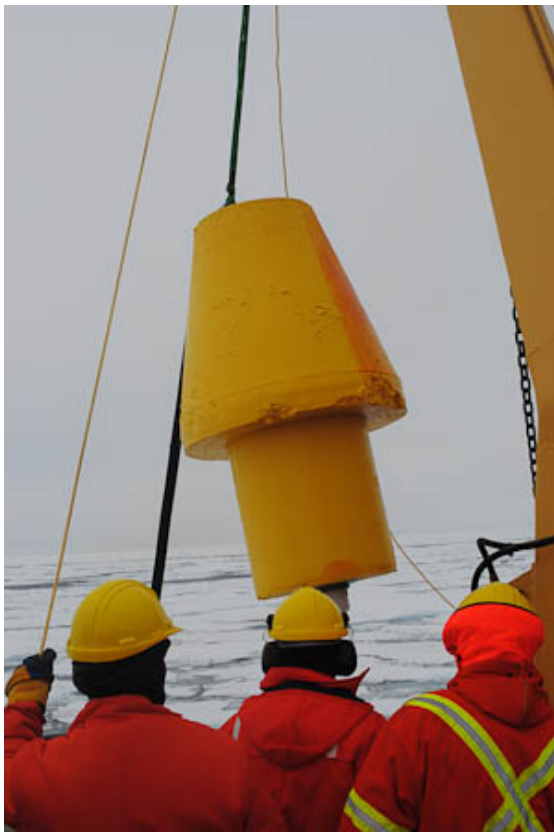
Crew members stand ready to guide the ITP to the deck. While ramming ice to break up floes, the hull of the ship scraped against the float, leaving a red stripe on its side.
