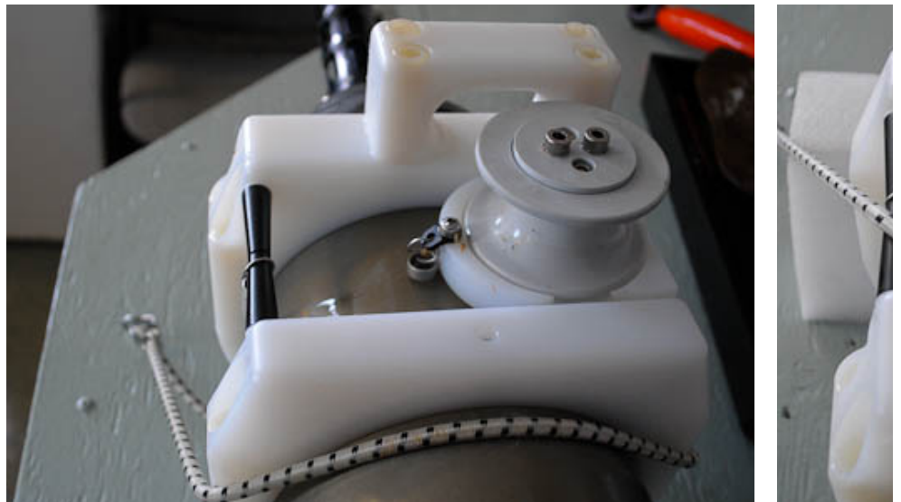
The right picture shows a fully functional wheel portion of the ITP with its spring intact. The left photo shows the float after colliding with a floe. WHOI engineers will account for this design flaw while developing the next generation of ITPs.
