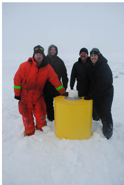
WHOI's "Buoy Boys" stand proudly next to the ITP. The white beacon atop the yellow float will transmit ocean profiles via satellite to Woods Hole laboratories. The profiles will then be posted online for public viewing.
