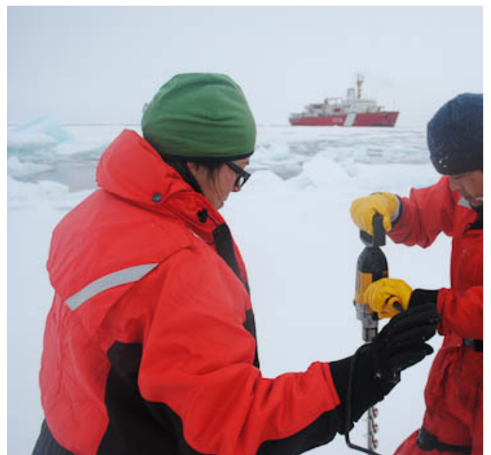
Orlich and Tateyama and drill to determine the ice's depth.
