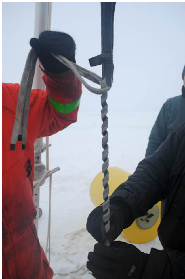
WHOI's Kris Newhall captures the ITP line in a "Yale grip." The Yale grip functions like a trap to stop the descent of the anchor so instruments can be attached to the line. Like its namesake, the grip is strong, trustworthy, and very attractive.
