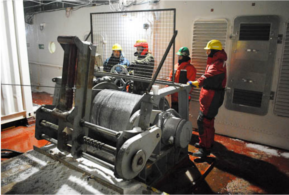
Kelly Young and Jeff Charters monitor the winch while deploying a rosette cast by Seaman Barney Noseworthy.
