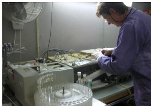
Rick Nelson loads a sample on the the gas chromatograph for CFC analysis. The sample has to be analyzed right away to minimize air contamination.
