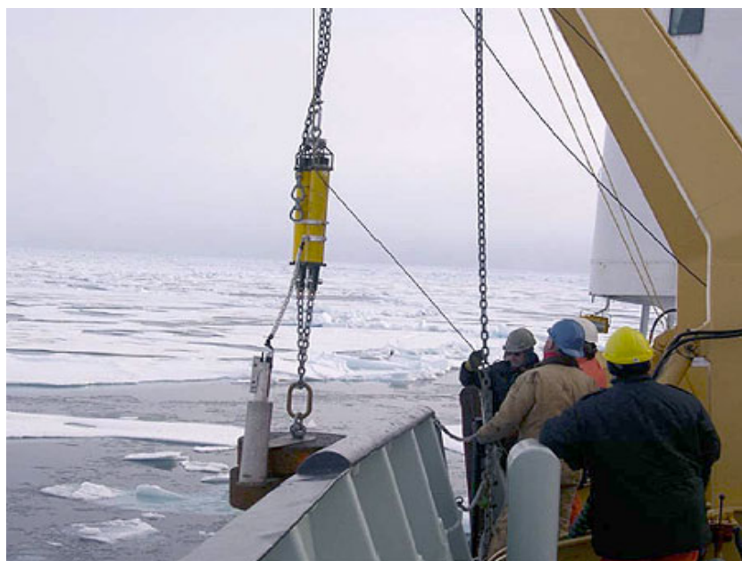
Figure 9. Lowering the anchor, BPR, and releases during anchor first mooring redeployment.
