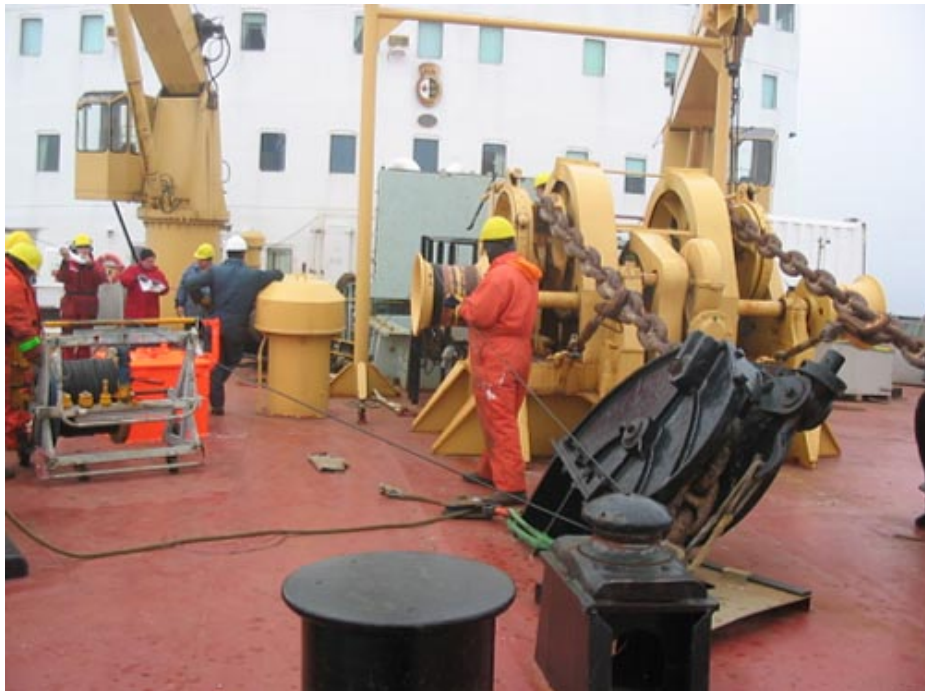
Figure 11. Wire fairlead windlass capstan to tension cart.
