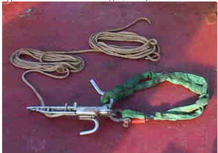
Figure 13. Brailer release hook and Lift All sling.
