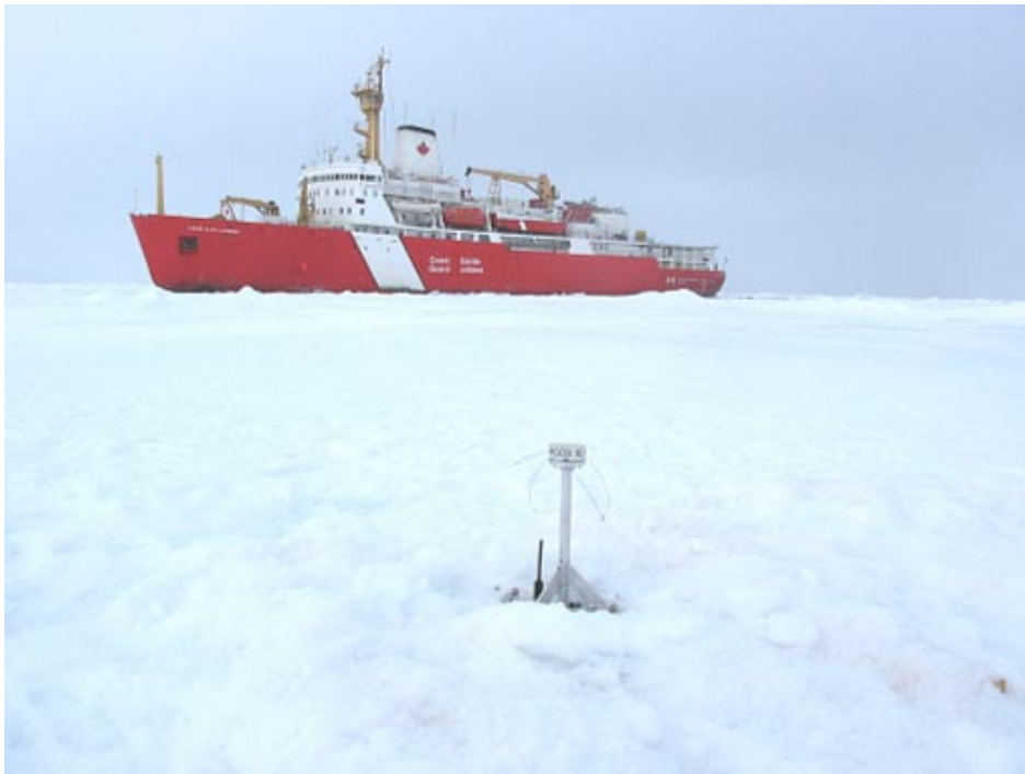
Figure 20. BGFE ice beacon deployed from CCGS Louis S. St. Laurent in summer 2003.
