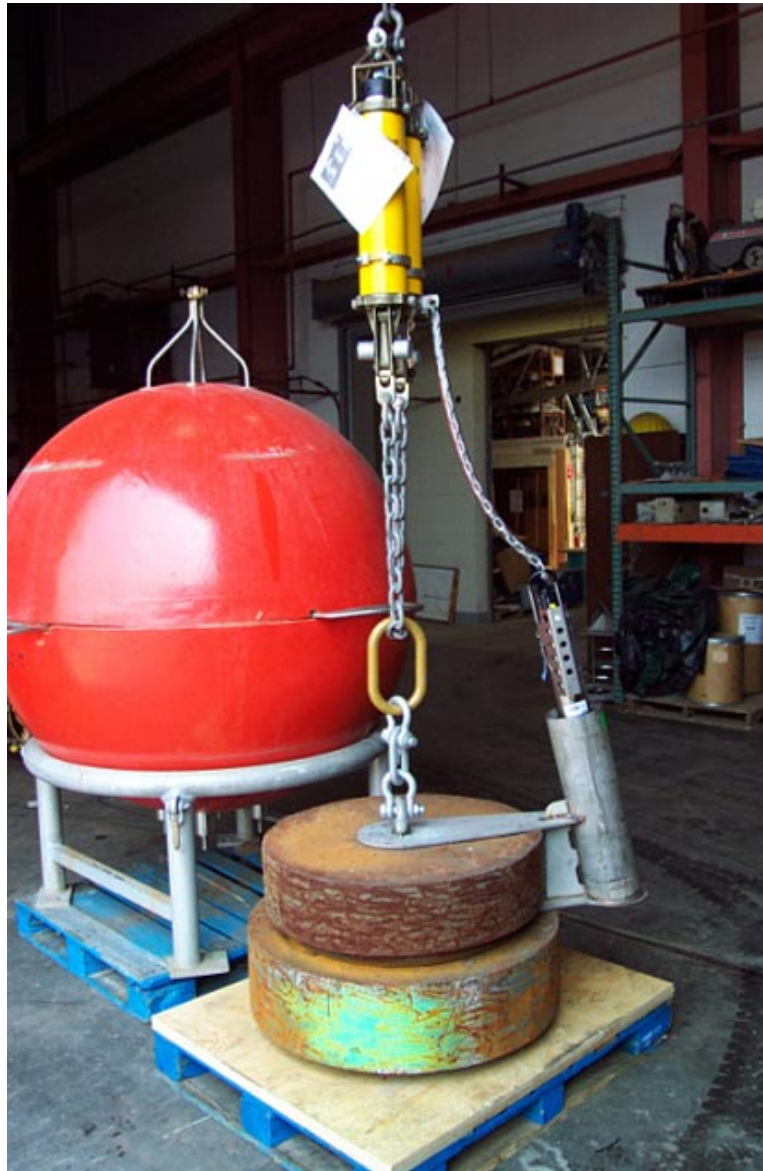
Figure 12. BGFE mooring anchor, SeaCat recorders and dual release package
