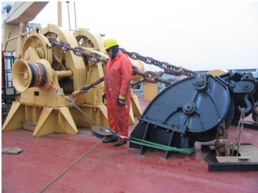
Figure 9. Fair lead block and stopper line
