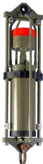
These are single point current meters using acoustic Doppler current sensing techniques. Other normally recorded channels are Temperature and tilt. Current Inventory is 30 instruments.
