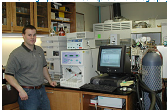
Sean Sylva prepares to use the High Performance Liquid Chromatograph (HPLC) to determine which organic compounds from an Archaea bacteria sample (collected at a Lost City hydrothermal vent) can be isolated and analyzed for ^{14}\text{C} .
