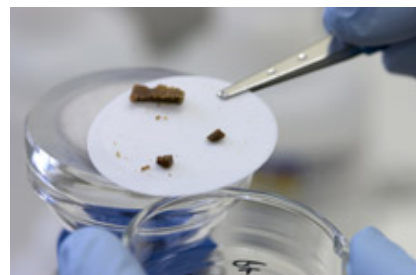
Transferring pre-treated wood on filter to a petri dish for drying.
