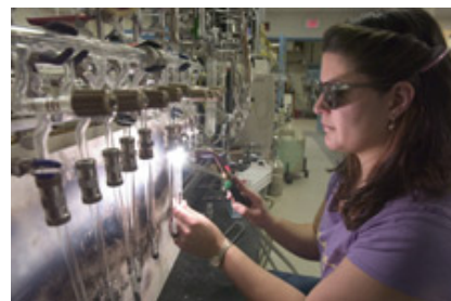
Mary Lardie flame-sealing organic carbon samples in combustion tubes on the vacuum-line system.
