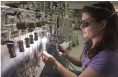
Mary Lardie Gaylord flame-sealing organic carbon samples in combustion tubes on the vacuum-line system.
