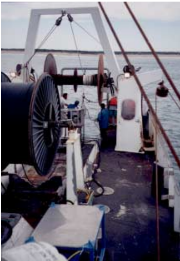
Fig. 3 Cable laying configuration on F/V Nobska shows conversion of fishing net drum pedestal for cable, cable tensioning engine at stern with arch easing cable beneath A-frame. Power system for cable engine sits next to fish hatch in foreground.
