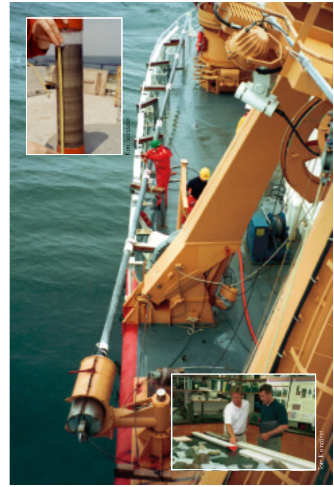
Seafloor sediment cores like the one at upper left provide a long, continuous record of changes in both the environment and types of organisms and species living in the marine ecosystem. The sediments are collected with corers like the one in the large photo. The corer is dropped vertically from the ship with the weight (foreground) uppermost to drive the core barrel into the mud. In lower photo, OCCI Director Bill Curry, at left, explains the value of sediment cores in climate studies to a congressional staff member at the WHOI Seafloor Samples Laboratory.
