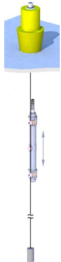
Figure 1: Schematic drawing (not to scale) of the WHOI Ice-Tethered Profiler (ITP) system.
