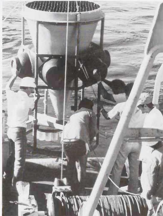
Figure 5. The Black Sea sediment trap on the stern of the research vessel.
