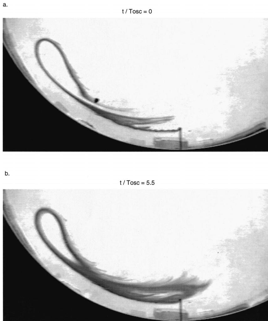
FIG. 5. Dye intrusion tracing the edge of the steady figure-eight gyre. The dimensionless times  $t/T_{osc} = 0$  and  $5.5$  correspond to 9 and 21 min after injection is begun. North is to the left and west is downward. The dye needle is shown as a thin line protruding through the western boundary.
