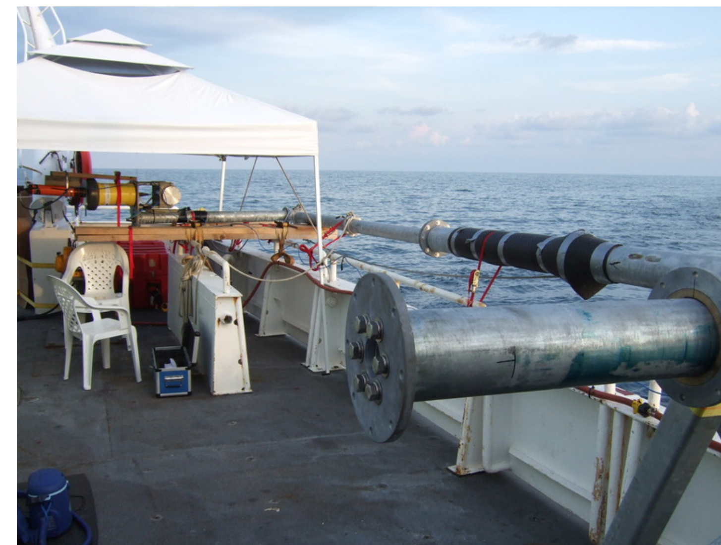
Figure 2: USBL pole system used by Jason and Sentry on ships of opportunity. In this case, Sentry was aboard Endeavor at the Deepwater Horizon site, June 2010.
