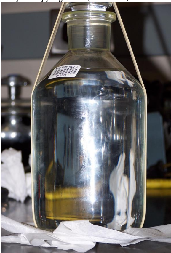
Figure 4. Stopper sealing technique. Apply pressure downward with a clockwise rotation to get grease to “fill” the joint properly. Joint should look “clear” with grease applied, ie no bubbles or wet streaks. Below is a picture of a properly sealed bottle ready to be placed in the sample shipping crate (AMS Box).
