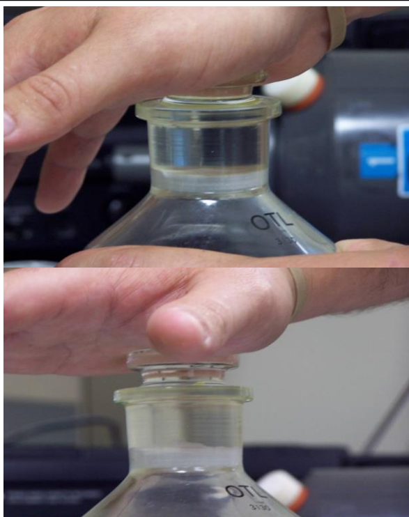
Figure 4. Stopper sealing technique. Apply pressure downward with a clockwise rotation to get grease to “fill” the joint properly. Joint should look “clear” with grease applied, ie no bubbles or wet streaks. Below is a picture of a properly sealed bottle ready to be placed in the sample shipping crate (AMS Box).
