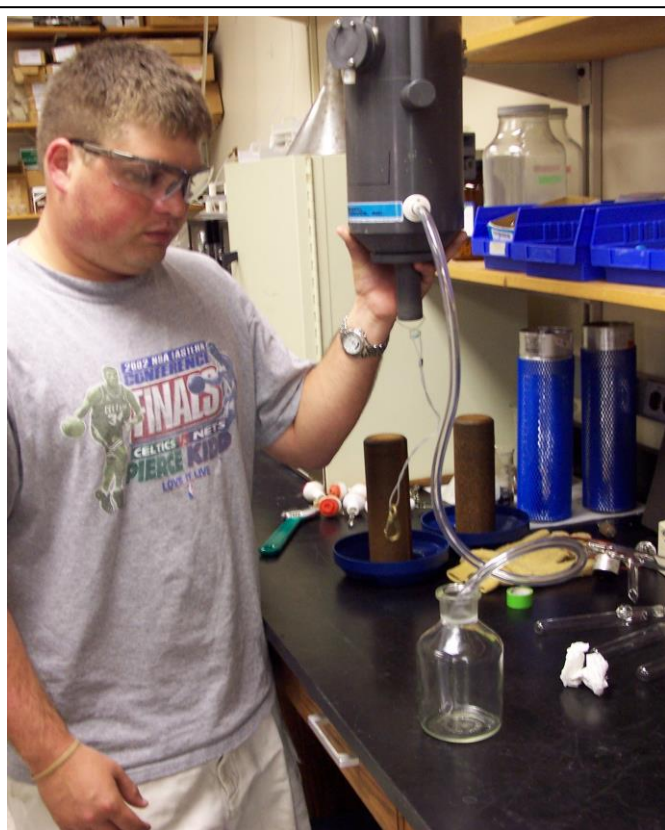
Figure 1. Filling bottle from Niskin. Note the tygon tube is in the base of the bottle. Count how long it takes for the bottle to fill, and then double the time to allow the water to overflow the bottle. Pull out the tygon tube, and spill out enough water to leave an approx. 3/8" head space below the stopper joint.
