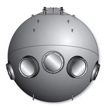
✓ The new sphere will have five, rather than, three viewports; the forward-looking viewports will be 7, rather than 5, inches in diameter. To withstand pressures at greater depths, the sphere will be 3, rather than 2, inches thick, with an interior diameter that is 4.6 inches wider than *Alvin's* current sphere. That increases the interior volume by 18 percent, from 144 to 171 cubic feet.
