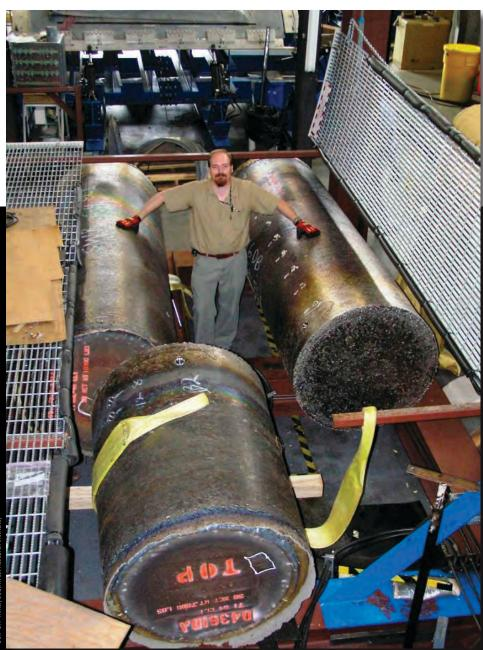
▲ Titanium used to forge the new personnel sphere started out as barrel-shaped ingots fabricated by a mill in Pennsylvania. The two larger ingots, each weighing 17,000 pounds, were shaped into hemispheres that were joined to create the crew compartment. The third ingot, weighing 7,000 pounds, will be used to make viewport and hatch inserts.
