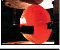
At a forging plant in Wisconsin, the titanium ingots were heated to 1,700°F and "edge rolled" to get it them as close to circular as possible. Next, they were paddled to flatten them and to reduce their thickness to about 6 inches.
