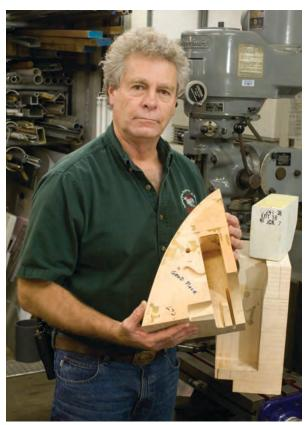
▲ WHOI engineer Rod Catanach is overseeing the development of new syntactic foam, the material used to provide buoyancy that allows *Alvin* to float back to the surface. The foam is made of a matrix of billions of microscopic hollow glass spheres embedded in a hard epoxy. It must withstand the crushing pressure at depths of 6,500 meters, or 4 miles.
