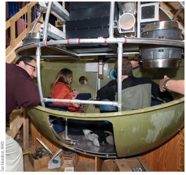
▲ Scientists test a mock-up of the new *Alvin* sphere constructed by engineers at Woods Hole Oceanographic Institution. They offered feedback on ways to make the sphere more comfortable and effective.
