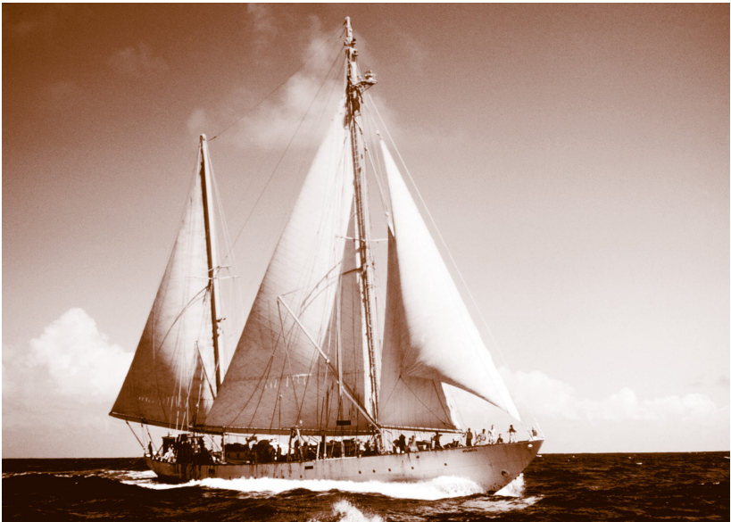
Bigelow applied knowledge gained on many research voyages in the Gulf of Maine to design of the first blue-water research vessel, the 142-foot steel-hulled ketch Atlantis.
