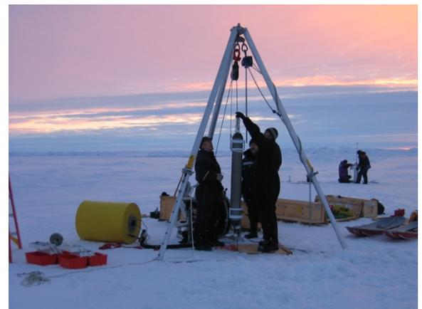
An Ice-Tethered Profiler being deployed during one of the AARI expeditions during the IPY.
