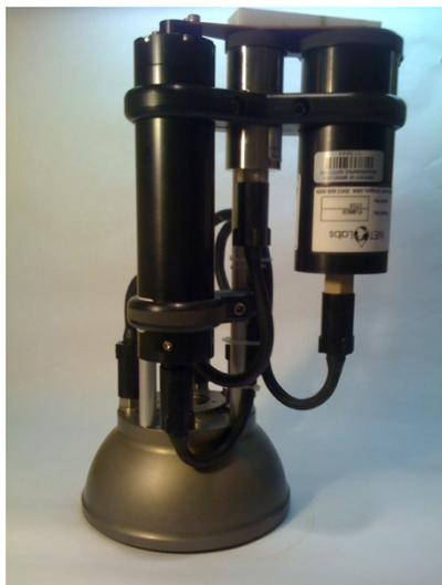
Photograph of the prototype bio-optical sensor system mounted on an ITP end cap.
