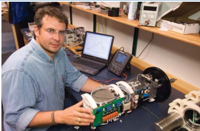
Rich Camilli in the lab with Gemini, his miniature mass spectrometer.
