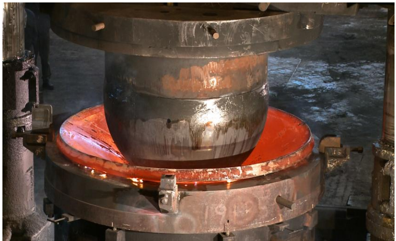
Figure 3.2 Forging of a hemisphere in June 2008
