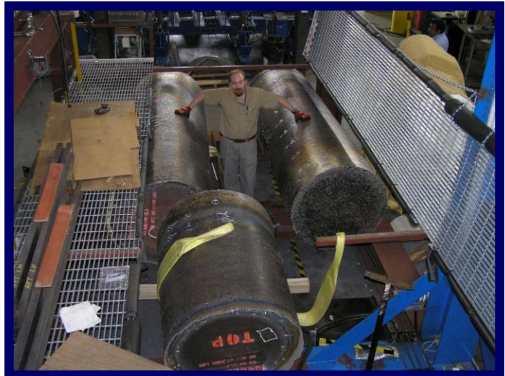
Figure 3.1 Two 36" hemisphere Ti alloy ingots and 1 insert ingot
