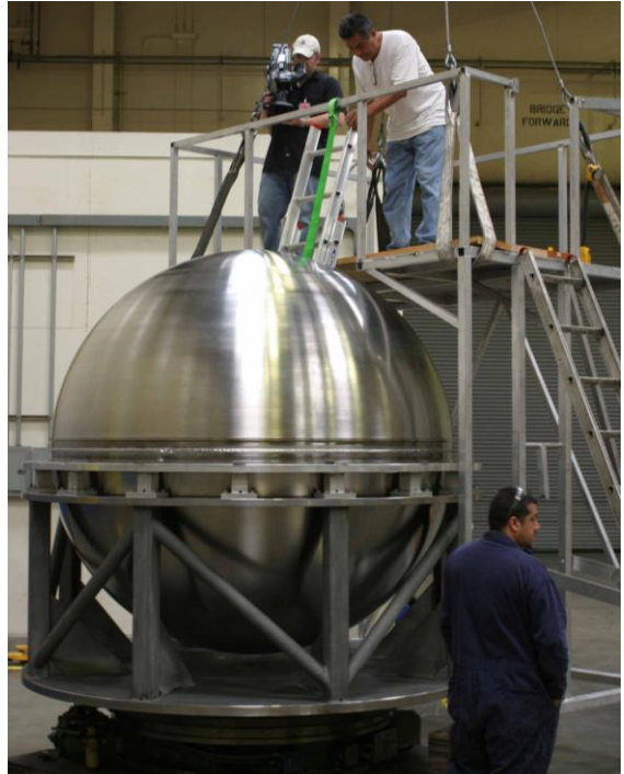
Figure 3.3 The sphere after a successful girth weld.
