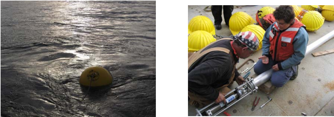
Figure 2 Deployment of the tube mooring for sampling the upper part of the water column. Left: the tube is visible floating behind the sphere. Right: Straneo and the Knorr's Boatswain assemble the tube mooring.
