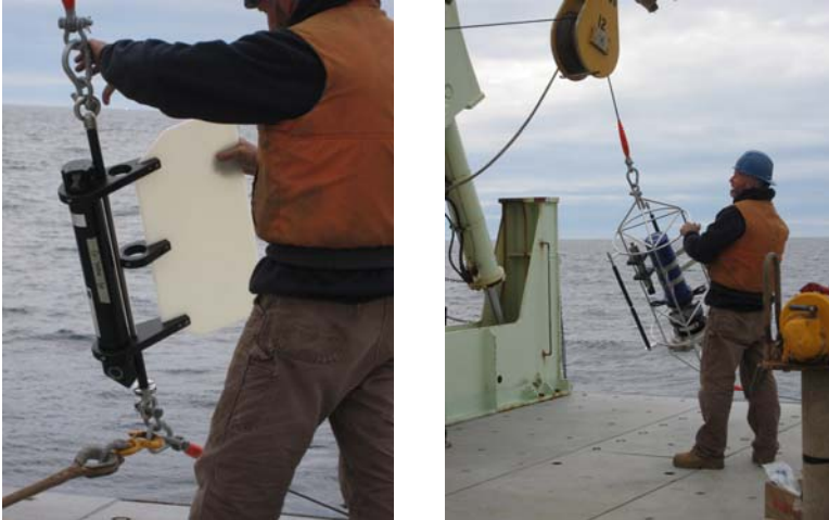
Figure 1: Deployment of velocity measuring instruments in Hudson Strait
