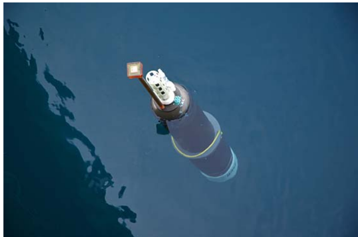
Figure 1: A polar profiling float drifts nose-up at various depths through the Arctic Ocean while measuring water temperature, salinity, dissolved oxygen and pressure. The floats are programmed to rise to the surface periodically and send data via satellite antenna to scientists on shore.
