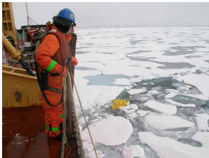
Figure 4: Recovery of sediment trap mooring from ice-covered waters in the Arctic Ocean during the August 2008 research cruise aboard the Louis St. Laurent (Photo courtesy of MIT/WHOI Joint Program student David Griffith). Note yellow “hard hat” floatation balls that have popped up in a gap in the ice made by the ship. The rest of the mooring is lying below, awaiting retrieval. All the moorings were successfully recovered and redeployed.
