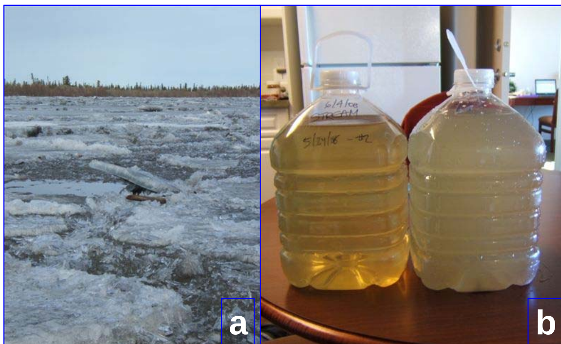
Figure 1: Photographs from sampling trip (May/June 2008) to the Mackenzie River Delta. (a) River just prior to break-up of the ice on the river; (b) water samples showing the high concentrations of dissolved (note color, left) and suspended (note turbidity, right bottle) materials carried by the river during this time period.
