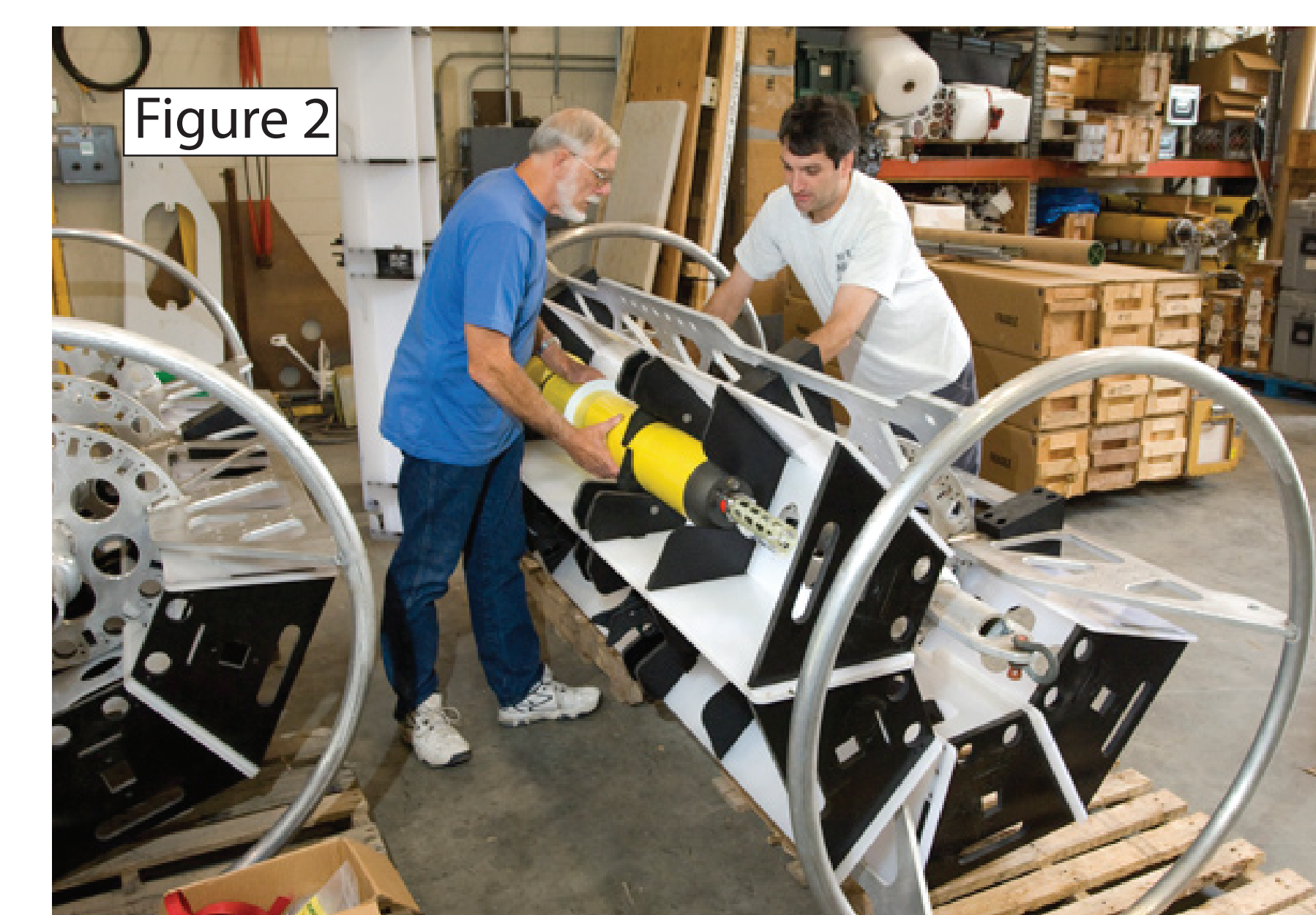
WHOI engineers Jim Valdes and Dave Wellwood load the Submerged Autonomous Launch Platform (SALP) with APEX floats (Figure 2). The prototype SALP is designed to launch floats when triggered by passing temperature and pressure anomalies, which indicate that an Irminger Ring is passing by the mooring. After release, the floats profile once every five days, and drift at a nominal 300 meter 'park depth'.
