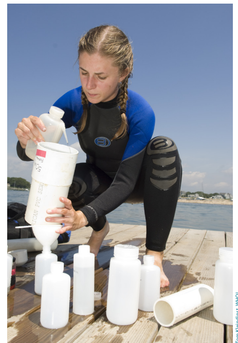
MIT/WHOI graduate student Christine Mingione rinses a plankton sample from a collection screen into a bottle. She will take the samples back to the lab to count the larvae and image them using polarized light.
