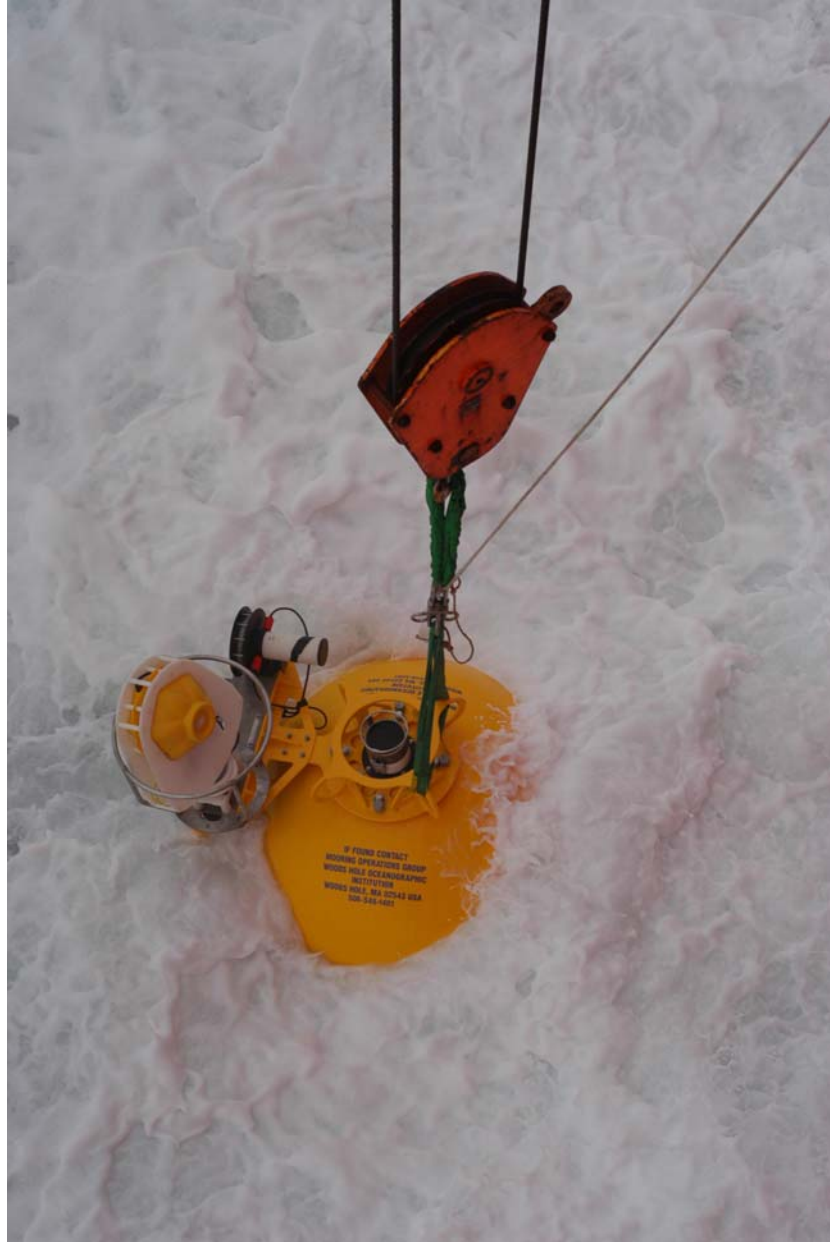
Figure 3: The top section of the monitoring mooring enters the water upon deployment. The frothing water is due to the ship’s underwater bubbleers that keep the area free of ice. The photograph was taken moments before the heavy rope (in green, attached to the ship’s crane) released the large yellow top float of the mooring. Once deployed, the top float resides at 40m depth, with the “Arctic Winch” (on the left-hand side) attached to it. The sensor suite of the Arctic Winch is contained inside the small yellow sphere, adjacent to the spool of nylon line (see text for details). The photograph was taken by C.A. Linder, who was the photo-journalist during the cruise (see www.whoi.edu/beaufortgyre for further information).
