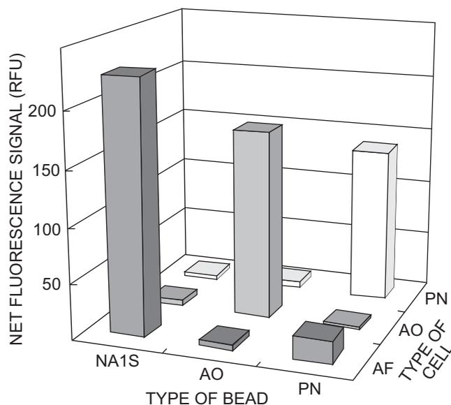
**Figure 3:** Net fluorescence signals from a multiplexed array containing probes specific for *A. fundyense* (NA1S), *A. ostenfeldii* (AO) and *P. australis* (PN) treated with cell lysates from each of the three species. Species abbreviations are 'AF' for *Alexandrium fundyense*, 'PN' for *Pseudo-nitzschia australis* and 'AO' for *A. ostenfeldii*
