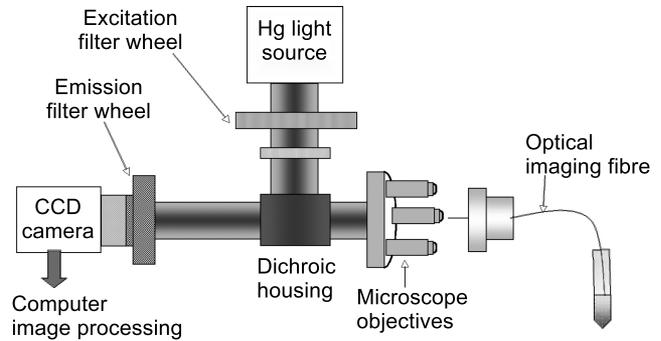
**Figure 1:** Schematic of the fibre optics instrumentation. Internal reflection allows both excitation and emission light to be carried in a single fibre
