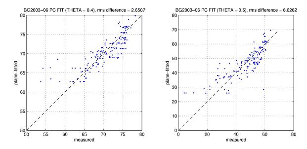
Figure 6. Scatter plot of observed potential conductivity from the icebreaker stations versus the plane fits to the data for the 0.4 °C (left) and 0.5 °C (right) potential isotherm surfaces. Shown are values in mmho x 1000.
