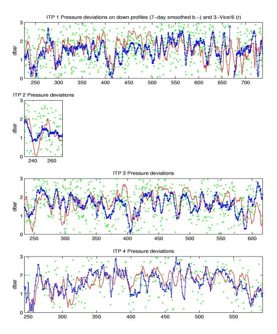
Figure 4. Observed differences between the estimated pressure of selected potential isotherms on up-going and adjacent down-going profiles (green points) versus profile number, and after smoothing with a 7-day low-pass filter (blue line). Shown with red line are modeled pressure offsets based on low-pass-filtered ice floe speed estimates. Results from ITPs 1-4 are shown (top to bottom).
