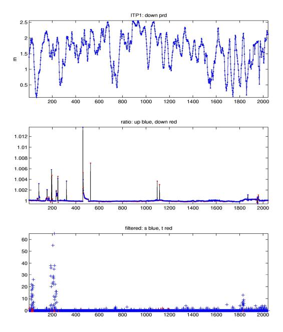
Figure 7. Top: Down-going pressure deviation correction (in db) for ITP 1 versus profile number estimated from ice-floe drift speed. Middle: Conductivity calibration factor for each ITP profile based on 2003-2006 summer icebreaker CTD stations. Bottom: Number of ITP 1 data spikes removed per profile based on final filtering routine. Blue indicates salinity points, red are temperature points.
