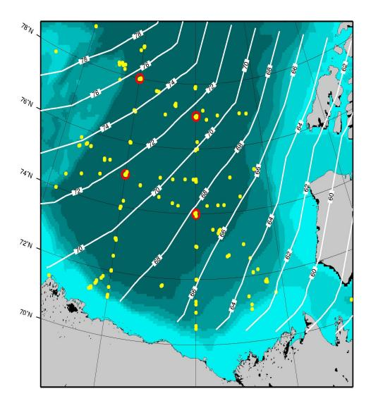
Figure 5. Potential conductivity estimated at the  $0.4~^{\circ}\text{C}$  potential temperature surface from all 196 CTD icebreaker stations collected between 2003 and 2006 (contours =  $1000~^{\circ}$  ([potential\_conductivity\_at\_0.4] - 29.2~mmho)).
