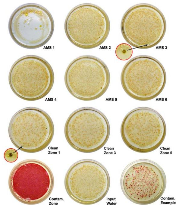
Fig. 7. Protection of samples from contamination after exposure of the AMS nozzle to a 1 × 10<sup>6</sup> viable cells ml<sup>-1</sup> seawater suspension of *S. marinorubra*.
