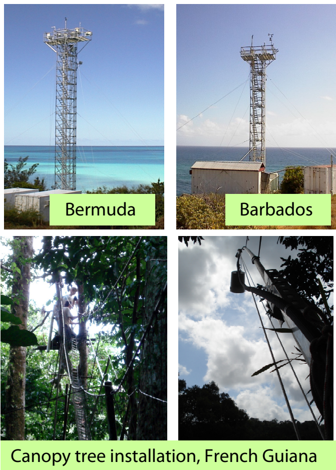
Figure 1. Atmospheric sampling towers at Bermuda and Barbados, and portable aerosol sampler installation in Amazon rainforest canopy tree in French Guiana. Typical HiVol aerosol samplers are used for the tower sampling. Left photo shows mounting the sampler on the canopy platform and the cabled walkway in French Guiana. Vacuum hose leads to the pump house at the end of the walkway. Bottom right photo shows flagpole designed to raise and lower filter holders (located under rain shield in photo) to change the sample filters.
