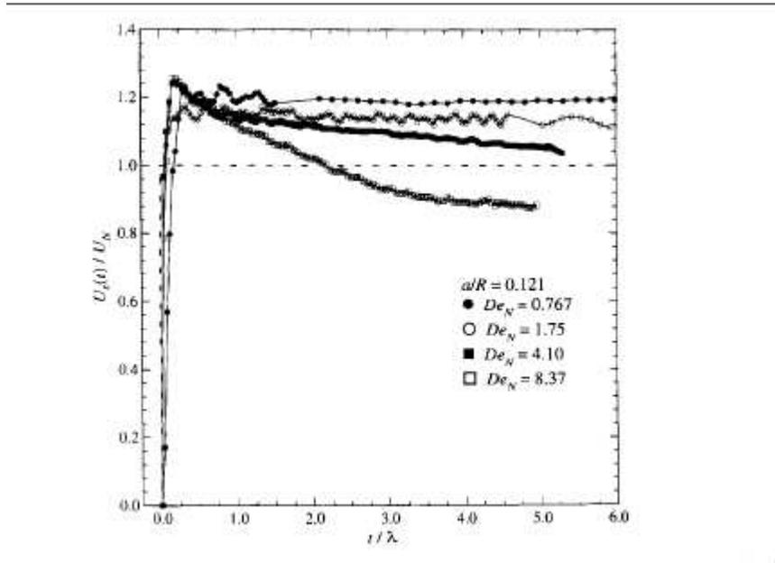
Figure 10: Velocity of the sphere plotted against time
