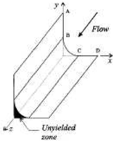
Figure 15: Unyielded zone in the corner of a rectangular channel.
